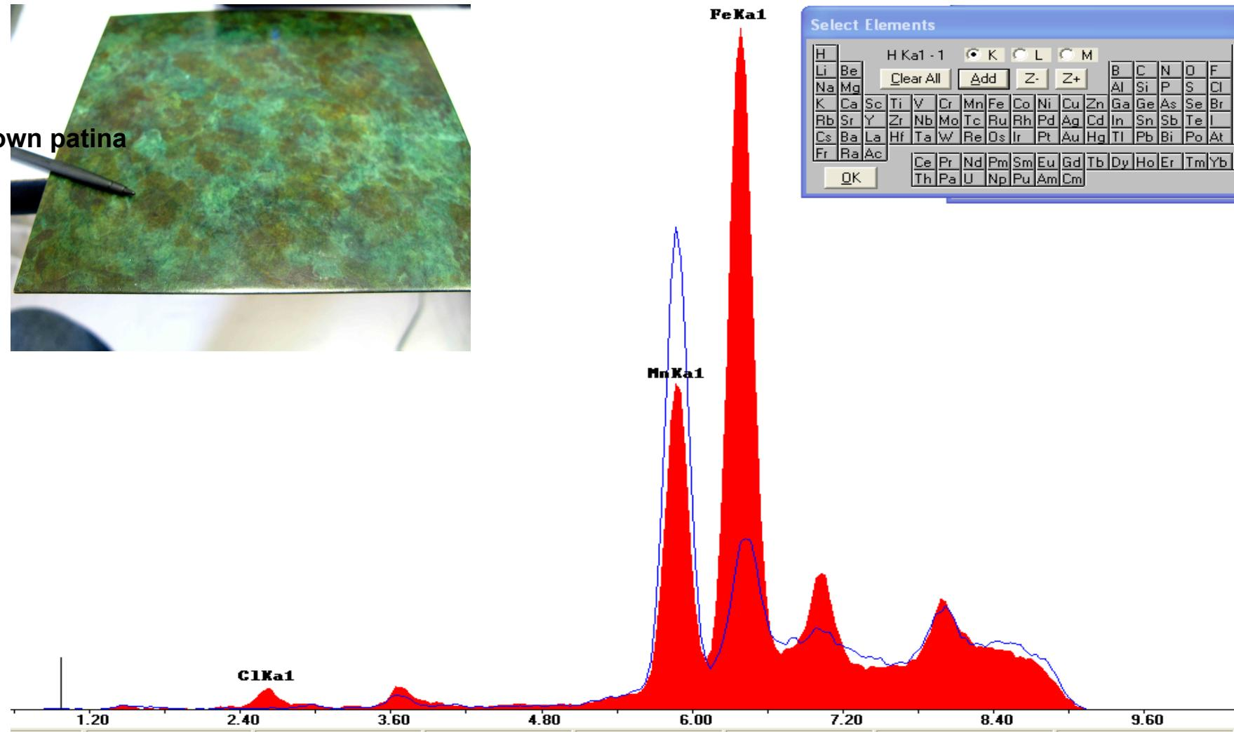
**patina brownSI1 (red) /Cu SI1 (blue):** Cu SI1 is the polished spot on the back of the plate, pure alloy. It is clear that the patina contains a large amount of Fe and some Cl. The red spectrum is the brown patina spot shown in the above picture.
