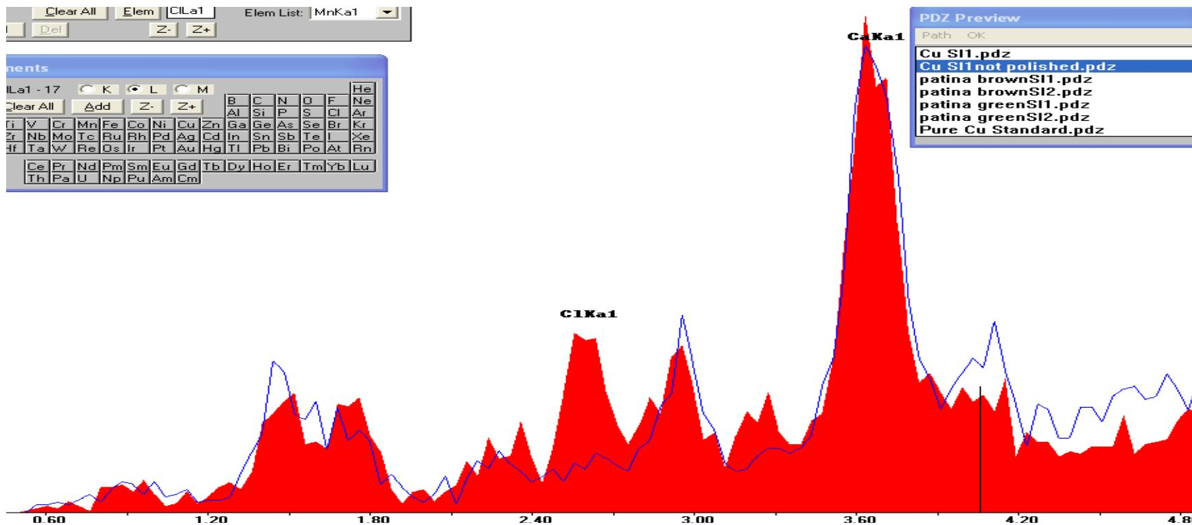
The **red** spectrum is the unpolished back side of the SI Cu plate. The **blue** spectrum is the polished spot on the back side of the SI Cu plate. One can see that the unpolished surface shows a trace of Cl.
