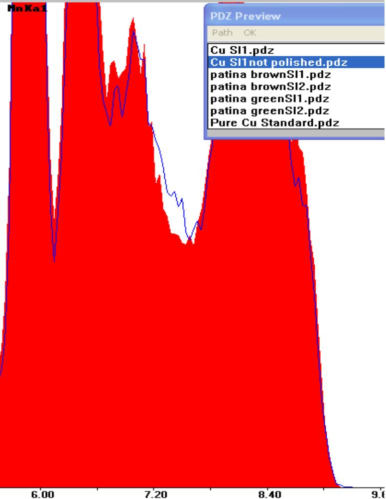
The red spectrum is the unpolished back side of the SI Cu plate. The blue spectrum is the polished spot on the back side of the SI Cu plate. One can see that the unpolished surface shows a trace of Cl. The next slide shows the Cl on an expanded scale.
